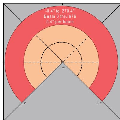
Fig. 4-1 Beam Report Selection Mask, All Beams
