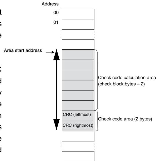
Calculate and write the check code using the Memory Check command (MD) after writing data and verify the check code before reading data. This enables detecting in advance data corruption in Tags that can occur while the Tags are not being accessed.
