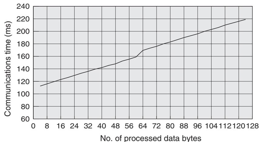
Read and write communications with Tags is performed in 4-byte units. This means that the communications time can be minimized by specifying the address and number of bytes so that the write start address is a multiple of 4.
