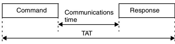
The TAT is the total processing time required to operate the CF Reader/Writer, from the viewpoint of the Handy Terminal. The communications time is the time required for communications between the CF Reader/Writer and a Tag, and does not include communications with the host device.
