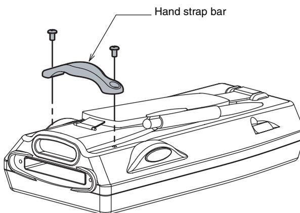
3. Insert the pin as shown in the following diagram to attach the hand strap to the Protective Cover.
