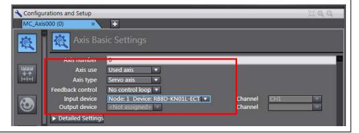
Make the Unit Conversion Settings according to the mechanical configuration. 4 Unit of display: mm Command pulse count per motor rotation: 1048576 pulse/rev Work travel distance per motor rotation: 10 mm/rev Configurations and Setup Unit of display
