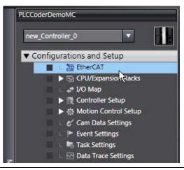
2 Drag the R88D-KN01L-ECT from the Toolbox to the master.
