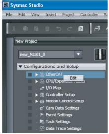
Right-click the EtherCAT master that is displayed in the Edit Pane and select Write Slave Node Address.
