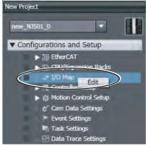
2 Select the I/O port on the I/O Map Tab Page and enter the variable name in the Variable column.
