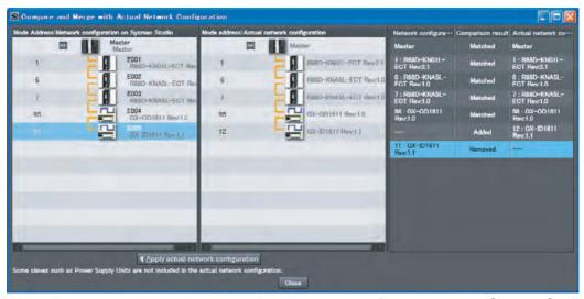
Here, either correct the node address in the network configuration on the Sysmac Studio or the node address in the physical slave in the actual network configuration, and then repeat the compare and merge operation to confirm that the configurations are the same.
