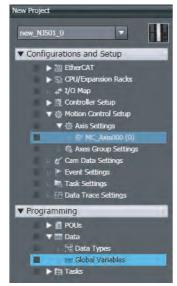
You can confirm that the MC\_Axis000 Axis Variable has been added automatically.
