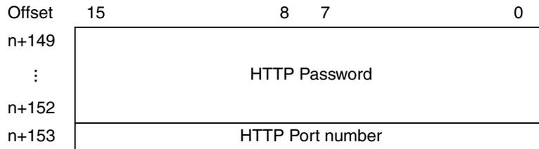
If the password for accessing the Ethernet Option Board's Web page is forgotten, find out it in this area. It is written in ASCII format.
