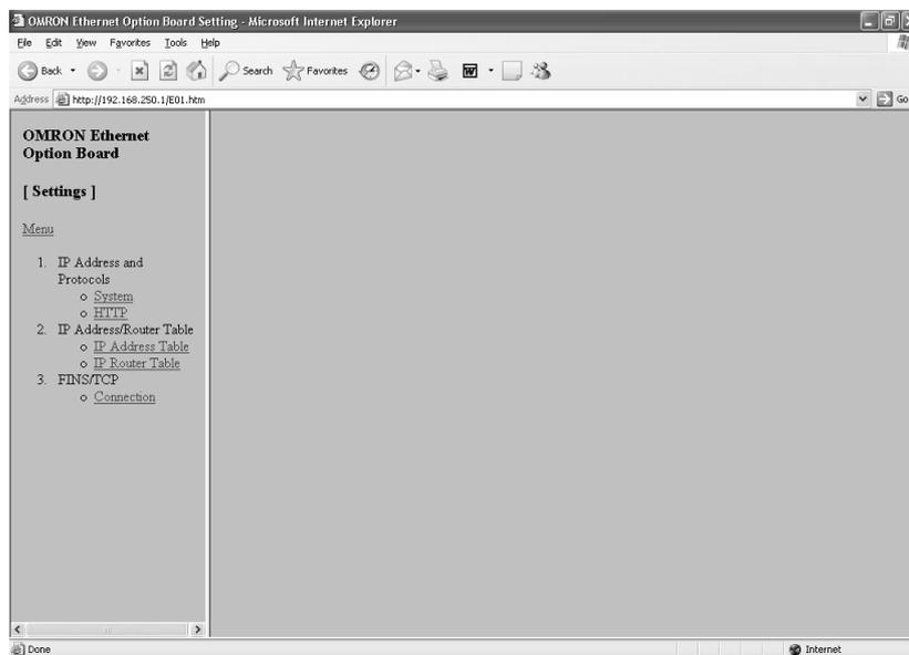
4. Select **1. IP address and Protocols - System** to display System menu.
