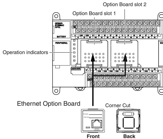
**Note** Only one CP1W-CIF41 can be mounted in one CP1L and CP1H PLC. If two CP1W-CIF41 Ethernet Option Boards are mounted in the PLC, the CP1W-CIF41 mounted on Option Board slot1 (left side) will run in abnormal status and ERR indicator will be ON. If the ladder program operates the with CP1W-CIF41 fatal error, the PLC will generate the non-fatal error.
