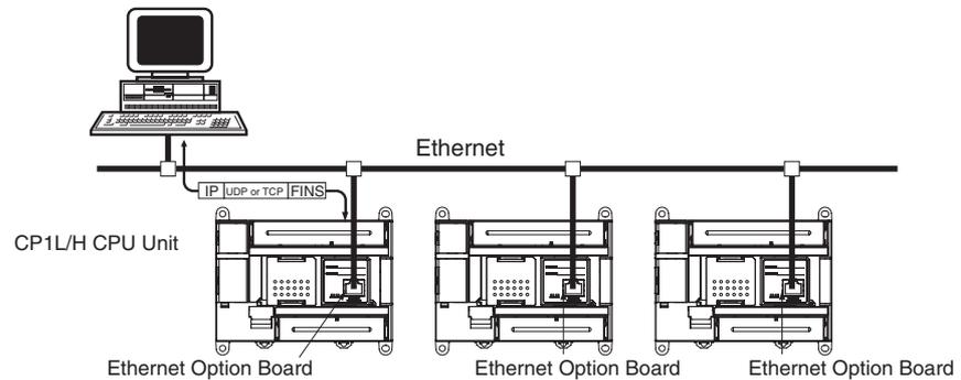
Executing, from the host computer, FINS commands with UDP/IP or TCP/IP headers enables various control operations, such as the reading and writing of I/O memory between PLCs, mode changes, and file memory operations.
