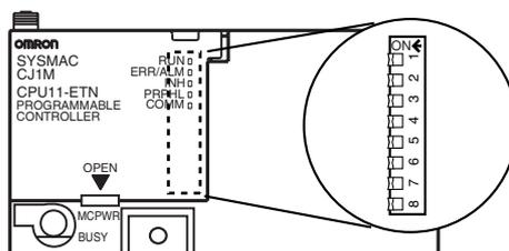
**Note** The language displayed for the CJ-series CPU Units is not set on the DIP switch, but rather is set using Programming Console keys.
