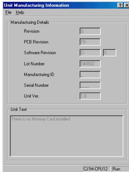
Use the above display to confirm the unit version of the Ethernet functional element connected online.
