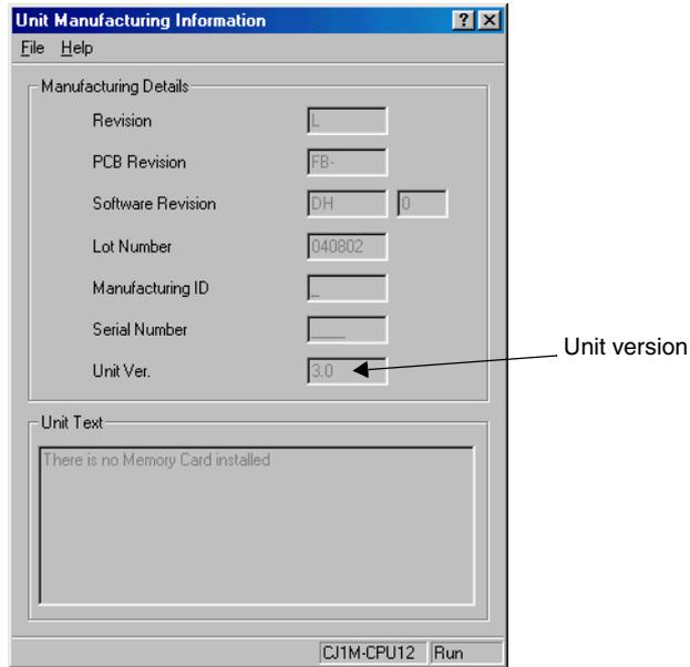
Use the above display to confirm the unit version of the CPU functional element connected online.
