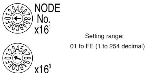
The top switch sets the sixteens digit (most significant digit) and the bottom switch sets the ones digit (least significant digit). The node address is factory-set to 01.
