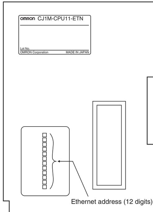
**Note** The Ethernet address can also be checked using the FINS command.
