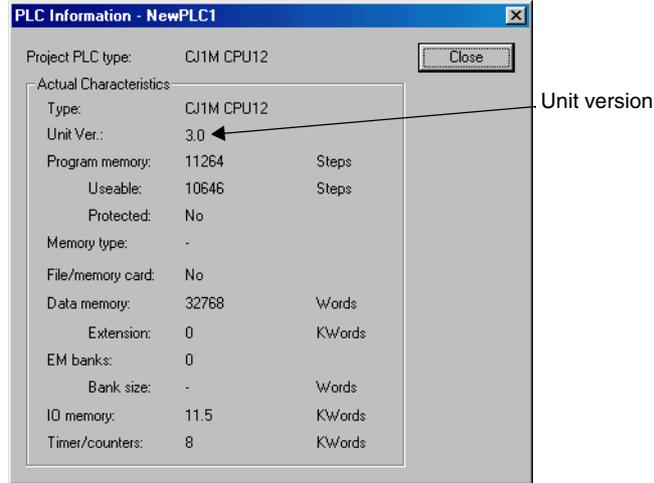
Use the above display to confirm the unit version of the CPU functional element.
