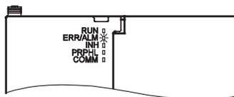
When the ERR/ALM indicator flashes, connect a Programming Console to the peripheral port and read the error message. If the message “BATT LOW” appears on the Programming Console\* and the Battery Error Flag (A40204) is ON (see note 1), first check whether the battery is properly connected to the CPU Unit. If the battery is properly connected, replace the battery as soon as possible.
