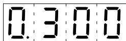
CIO 0300 Indicates that the first word on the Slave Rack is CIO 0300.
