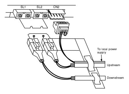
The SL1 connection of each node should be connected to the SL2 connection of the adjacent node. Likewise, the SL2 connection should be connected to SL1.
