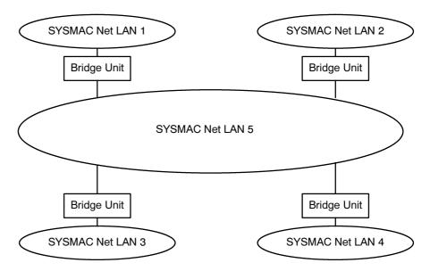
Again, each SYSMAC Net loop requires its own Line Server Unit to generate and monitor that loop's token. The routing table established at each of the Bridge Units sets the communication path between network loops. This is discussed in the next section.
