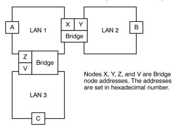
If node A of LAN 1 wants to communicate with node B of LAN 2, three processes occur in the exchange. First, node A sends information to X, the Bridge's node address on LAN 1. Then node X transfers the information to node Y, the same Bridge Unit but a different LAN loop. Finally, node Y transfers the information to node B. The response is then directed back to the sending PC along the same path.
