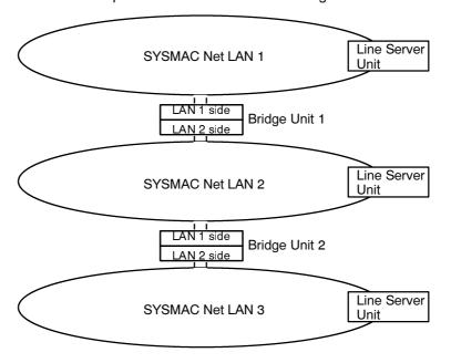
An AT-compatible computer equipped with a Net Support Board is required to set the Unit's network address and the routing tables. Once this information has been set, switch the initialization switch OFF and turn the power OFF and ON again.
