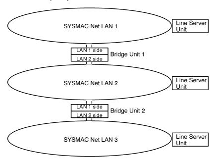
Network loops do not need to arranged linearly, as in the above configurations. They may also be arranged as the following figure indicates:
