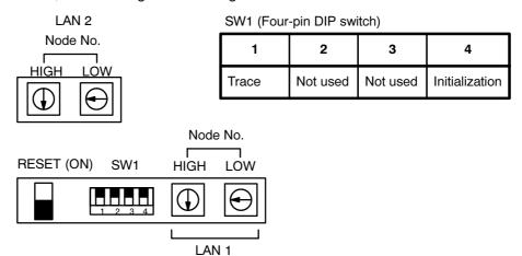
When the trace switch is ON, a record of transmission and reception through the Unit is stored and may be examined by performing a memory dump from a computer node on the network. The trace switch should be set to OFF, unless troubleshooting, since this slows the Unit's performance. For information regarding performing a memory dump, refer to the Net Support Board Operation Manual.
