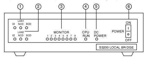
1. LAN1 Monitor LEDs Indicates connection status of LAN1
