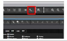
Select "PageDisplayed" for Events and select " SetVariable" for Actions. Enter "HMI\_IAG\_Axis\_Status.Fun ction\_Flg" for Variable and enter the number corresponding to the
