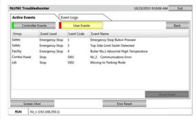
7. As described in Step 3, if you press the "Show Specified Page" button in the Details screen of the user event, the page created with Sysmac Studio can be displayed. You can specify the page from [HMI]-[Controller Events]-[User Events] on Sysmac Studio, as described in Step 8 below.
