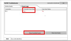
The screen is switched to "Controller Events". A list of the controller events that have occurred so far is displayed. Select an event from the list and press "Show Detail" at the right bottom of the screen.
