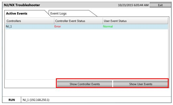
To confirm the contents of the currently raised errors, select the controller (to highlight it light blue) and press either "Show Controller Events" or "Show User Events".
