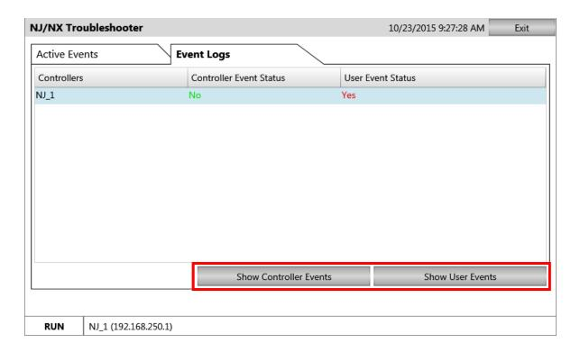
To confirm the contents of the errors that have been raised so far, select the controller (to highlight it light blue) and press either "Show Controller Events" or "Show User Events".
