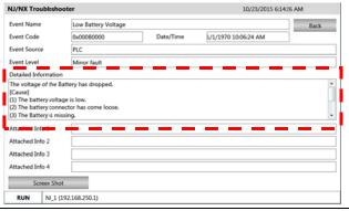
4. In Steps 2 and 3, if you press the "Screen Shot" button, the currently displayed screen can be captured and saved in an SD Memory Card. You can attach the saved image to defect reports.
