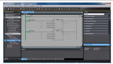
7. Enter the "Event Code" number that is set in "Event Settings" in "AlarmNumber" or "InfoNumber", and set "AlarmSetTrigger" or "InfoSetTrigger" to True. The corresponding error appears on the NA.
