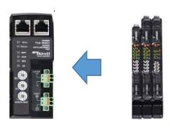
After attaching the Sensor Amplifier Units, connect the EtherCAT port of NJ to the "IN" side of the E3NW-ECT port with an EtherNet cable.
