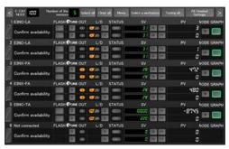
Displays the status of the sensor amplifiers connected to the E3NW-ECT Communication Unit.
