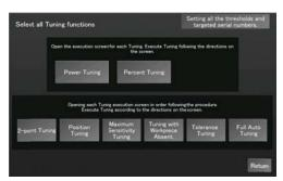
Executes each tuning to the multiple sensor amplifiers selected on the monitor screen at once.
