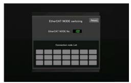
Displays a node No. to be monitored as well as a list of node No. connected to the Controller.
