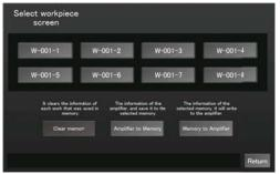
Reads and writes the status of all the sensor amplifiers, which are connected to the E3NW-ECT Communication Unit, into 8 memory areas.
