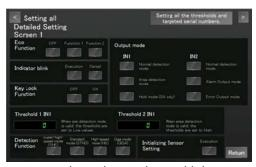
Executes each setting to the multiple sensor amplifiers selected on the monitor screen at once.
