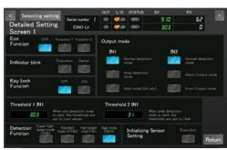
Displays and sets the status of each function to the selected sensor amplifier.
