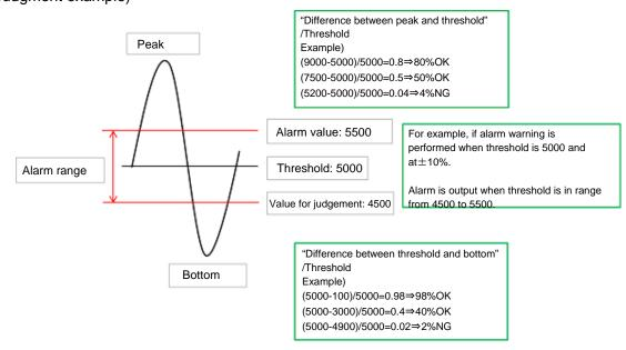
$^{\star}$  Once the above condition is met even for a short time, alarm is output but the error status is not maintained.
