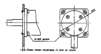
Note) Flange can withstand a static load up to 25 kg applied to the body of the resolver.
