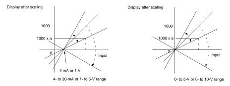
Example: When adjusting the factory set value 800 to a scaling value of 4200 Adjust the scaling while applying an actual input.
