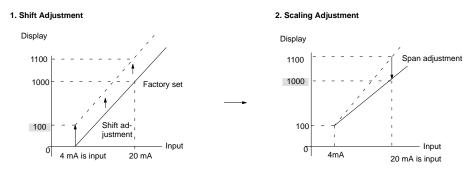
**Note:** 1. At the time of scaling adjustment, the starting point for changing the inclination of the straight line will be the minimum value of the input range. Therefore, when using only a part of the input range, repeat shifting and scaling adjustments several times.
