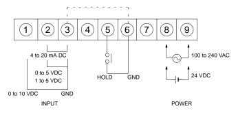
**Note:** Terminals 3 and 6 are connected internally. The power supply terminals are insulated from other circuits. **Connection Example with Inverter**
