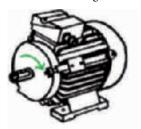
If motor is rotating in CCW (counter clock wise), change channel A by B in the encoder wiring and two output phases.
