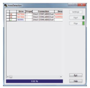
5. After detecting the inverter, automatically a new project will be created (in online mode) in the CX-Drive:
