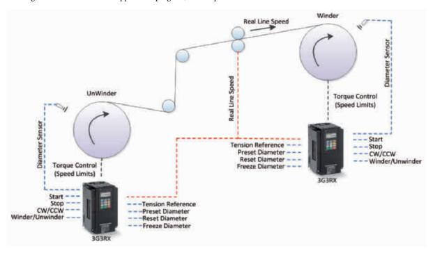
**Note:** In this specific Winder/Unwinder Application program, the tension set point is given through the analog input O and the diameter sensor through the analog input O2. Winder Line Speed Reference is forced internally in the firmware. It is needed to do a soft line acceleration ramp during winding/unwinding procedure.
