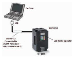
**3.** Use the CX-Drive autodetect function in order to go online with the 3G3RX inverter:
