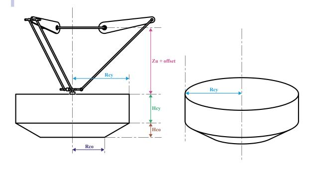
Zu + offset: -870 mm with rotational axis / -821 mm without rotational axis Distance from the Z-axis origin position to the tool flange
