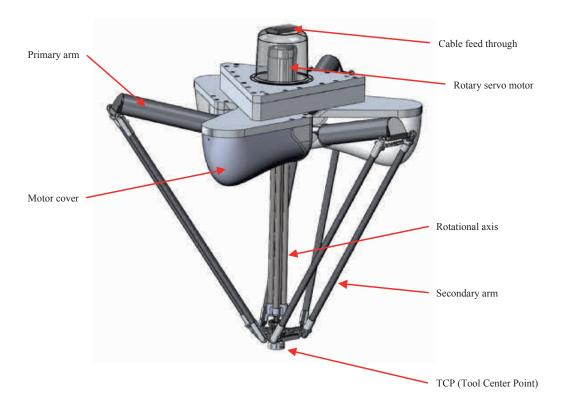
The CR\_UGD4\_XXLH robot consists of three radially placed axis which give the TCP freedom to move in three directions, X, Y and Z. An optional fourth axis can take care of the rotation, Rz, of the TCP.
