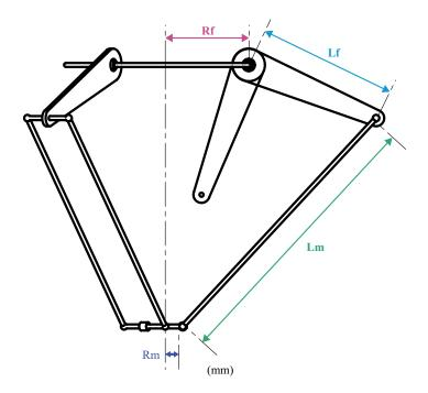
Rf: 147.5 mm Distance (radius) from the center of the fixed frame to the motor of the axis
