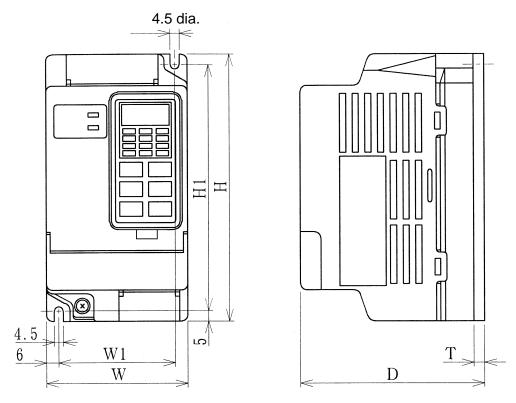
**Note 1.** For the 3G3EV-A2001M(-), 3G3EV-A2002M(-), and 3G3EV-AB001M(-), a U-shaped notch (4.5 mm wide) is provided instead of the upper mounting hole (4.5 mm in diameter).
