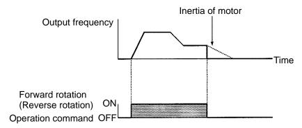
**Note** Do not input a RUN signal during a free-running stop if the motor's rotation speed is not sufficient slowed. If a RUN signal is input under these conditions, a main circuit overvoltage (OV) or overcurrent (OC) will be detected.
