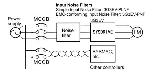
**Note** Use a noise filter designed for Inverters. A general-purpose noise filter will be less effective and may not reduce noise.
