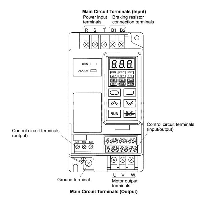
Note This diagram shows an Inverter with all terminal block covers removed.
