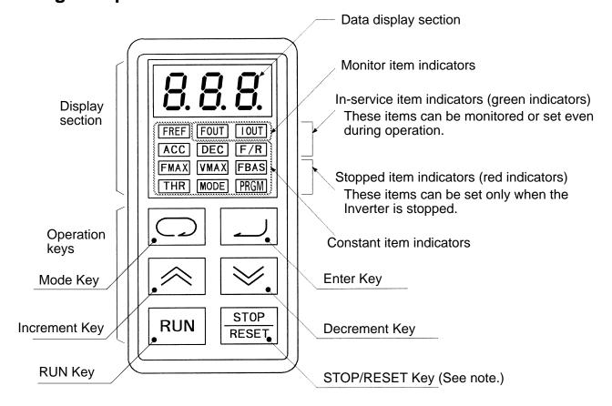
**Note** For safety reasons, the reset will not work while a RUN command (forward or reverse) is in effect. Wait until the RUN command is OFF before resetting the Inverter.
