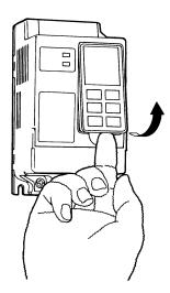
When the connector comes off, grip the lower edges of the Digital Operator, and slide it down until it comes off.
