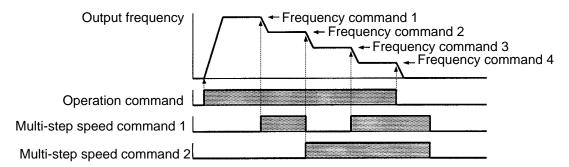
**Note** Multi-step speed command 3 is also used as the acceleration/deceleration time changeover command. When a frequency command (i.e., frequency command 5 to 8) turning ON multi-step speed command 3 is used, the Inverter will be in acceleration or deceleration operation with the constants set in n22 and n23 for acceleration and deceleration time 2.
