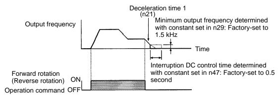
**Note** If the RUN signal is input again during a deceleration stop, deceleration will be stopped at the point of the input and acceleration will proceed at that frequency.
