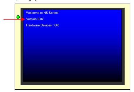
As the image above shows, the version of system program is displayed in the second line after turning ON the power. Check whether the version is changed to 2.0x.
