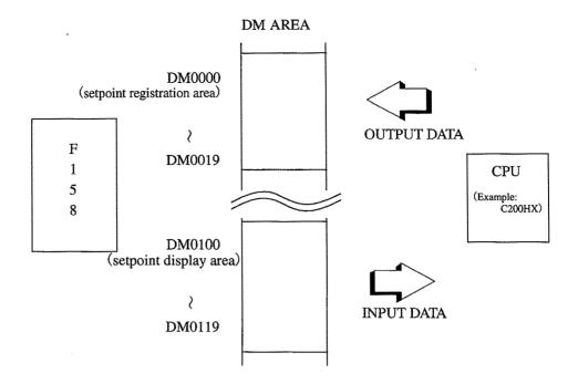
Example: For Machine No.0: 0000H is registered to DM1000 and 0100H is registered to DM1001 (C200H Series)
