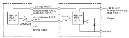
Note 1. The Encoder's data communication will stop when the main power supply goes OFF, but the Encoder's internal condenser and Receiver Unit's internal battery will supply power to retain multi-turn absolute data and measure rotational speed.
