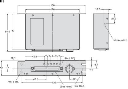
Note: OMRON 37-pin D-sub Connector XM2A-3701 (plug) (Order separately.) XM2S-3711 (hood) (Order separately.)
