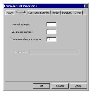
Select the Network tab, and set the Network number. The number must be other than 0 and unique. For SYSMAC LINK and Controller Link, the node number is set with the switch on the Support Board. Leave the other settings at the default values.
