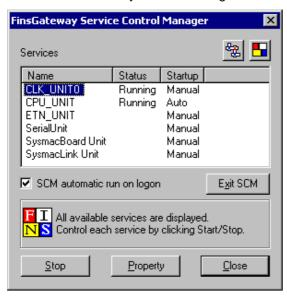
If the CLK\_UNIT does not start, follow through the Setting Up the Controller Link Support Board procedure again to solve the problem.
