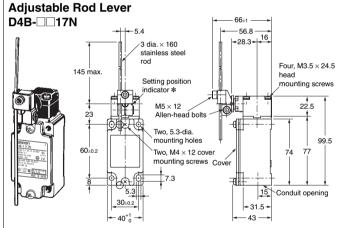
\* The lever can be set to any desired position by turning the operating position indicator.
