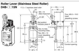
The lever can be set to any desired position by turning the operating position indicator.
