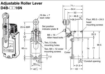
The lever can be set to any desired position by turning the operating position indicator.
