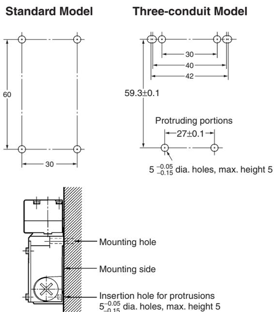
The D4BS can be mounted more securely by adding two protruding portions, each of which is 5 mm maximum in height and  $5^{-0.05}/_{-0.15}$  mm in diameter as shown below.
