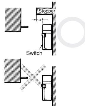
Refer to *Dimensions* for the mounting dimension of the Operation Key and mount the Operation Key correctly. The Operation Key will soon become damaged or worn out if it is not mounted correctly.
