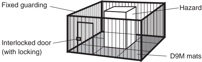
Figure 12 Note: Fixed guarding should meet the requirements of EN 953, EN 294, and EN 811.
