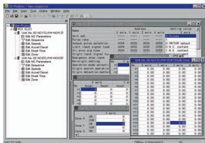
Note: The CX-Position transfers data in online communications with Position Control Units via FinsGateway. Either FinsGateway Version 2 or Version 3 Embedded Edition must be installed on the same computer as the CX-Position to enable online communications. (FinsGateway Version 3 Embedded Edition is provided on the same disk as CX-Position.) The communications method (i.e., the network type) depends on the FinsGateway driver that is used.
