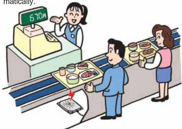
■ Simultaneous access to more than one Tag (1:N read/write)
