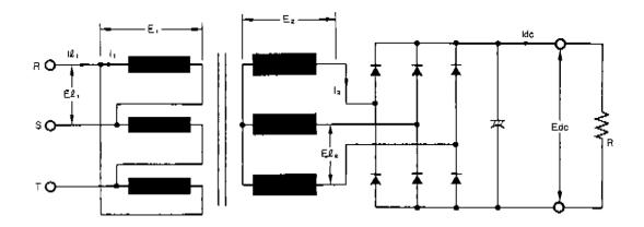
When 3-phase transformer is used, connect with  $\Delta$ -Y and Y- $\Delta$ . Connection to Y-Y causes imbalance of excitation.
