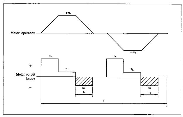
As shown above, regenerative energy occurs when motor output torque becomes negative. Regenerative energy in each section is given in the formula below:
