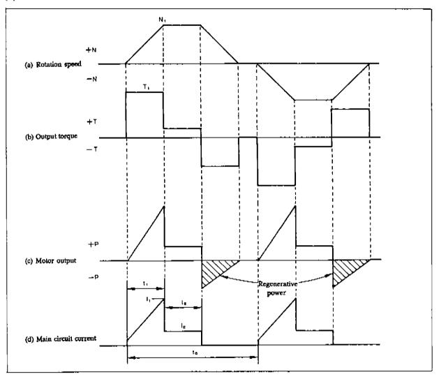
In case of horizontal installation of motor, the motor output at operation (a) in the figure above is given by the formula below:
