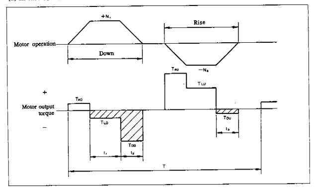
In the above movement, regenerative energy occurs while motor output torque becomes negative. Regenerative energies in each section is given by the formula below:
