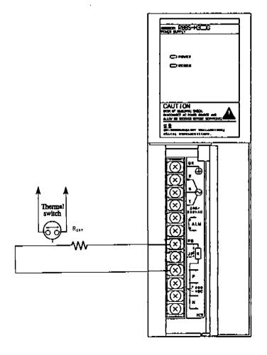
When you install an external regenerative resistance (REXT), remove a short bar between JP and RG terminals, and connect the external regenerative resistance between P and RG
