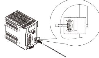
(3) Cleaning of the end face of the fiber connector of the sensor head side Remove the cap of the fiber connector, and wipe up and down the end face of the
